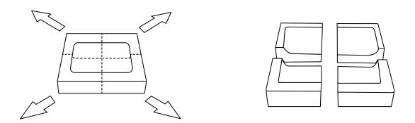
2. Place Corner Protectors at the bottom of the four corners of the tray before wrapping with sterilization wrap. Once in place, wrap the tray according to standard wrapping procedures.
